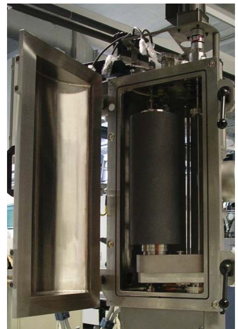
Fig. 2: LAM chamber with carbon cathode
