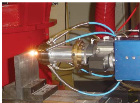
Fig. 2: Segmented powder nozzle for buildup welding in difficult positions
