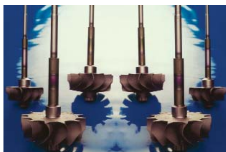
Laser beam hardened turbo charger shafts
