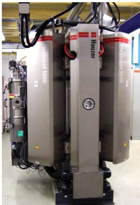
FlexiCoat® 1000 coating system made by Hauzer Techno Coating with integrated Laser-Arc module LAM400
