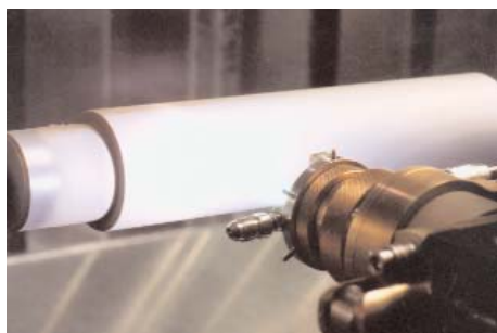
Plasma spraying of a shaft
