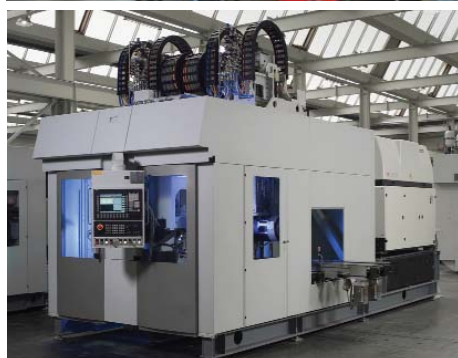
System for laser induction welding of hollow shafts (upper) and a welding process (lower) at GERTRAG Neuenstein (Manufacture EMAG Laser Tec)
