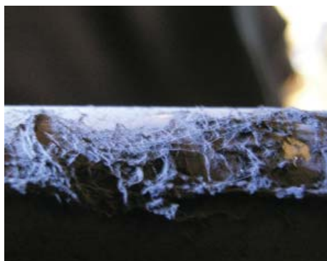
Fig. 1: Macroscopic webs consisting of strands of carbon nanotubes
