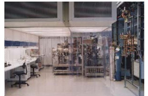
Device for the deposition of nano-meter multi-layers on large areas
