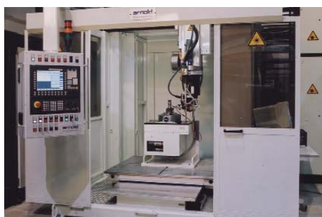
Laser beam welding system with 6 kW CO 2 high power laser
