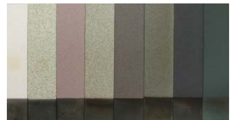
Fig. 2: Coloring due to different \text{Cr}_2\text{O}_3 fraction
