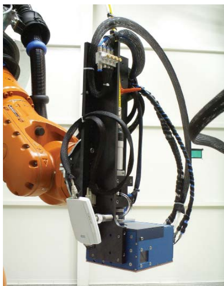
Fig. 2: Laser optics "LASSY", mounted to the robot
